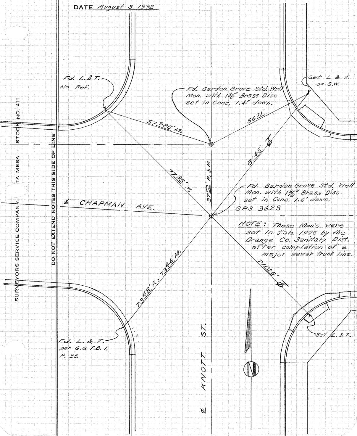
NOTE: These Mon's were set in Jan. 1976 by the Orange Co. Sanitary Dist. after completion of a major sewer trunk line.
