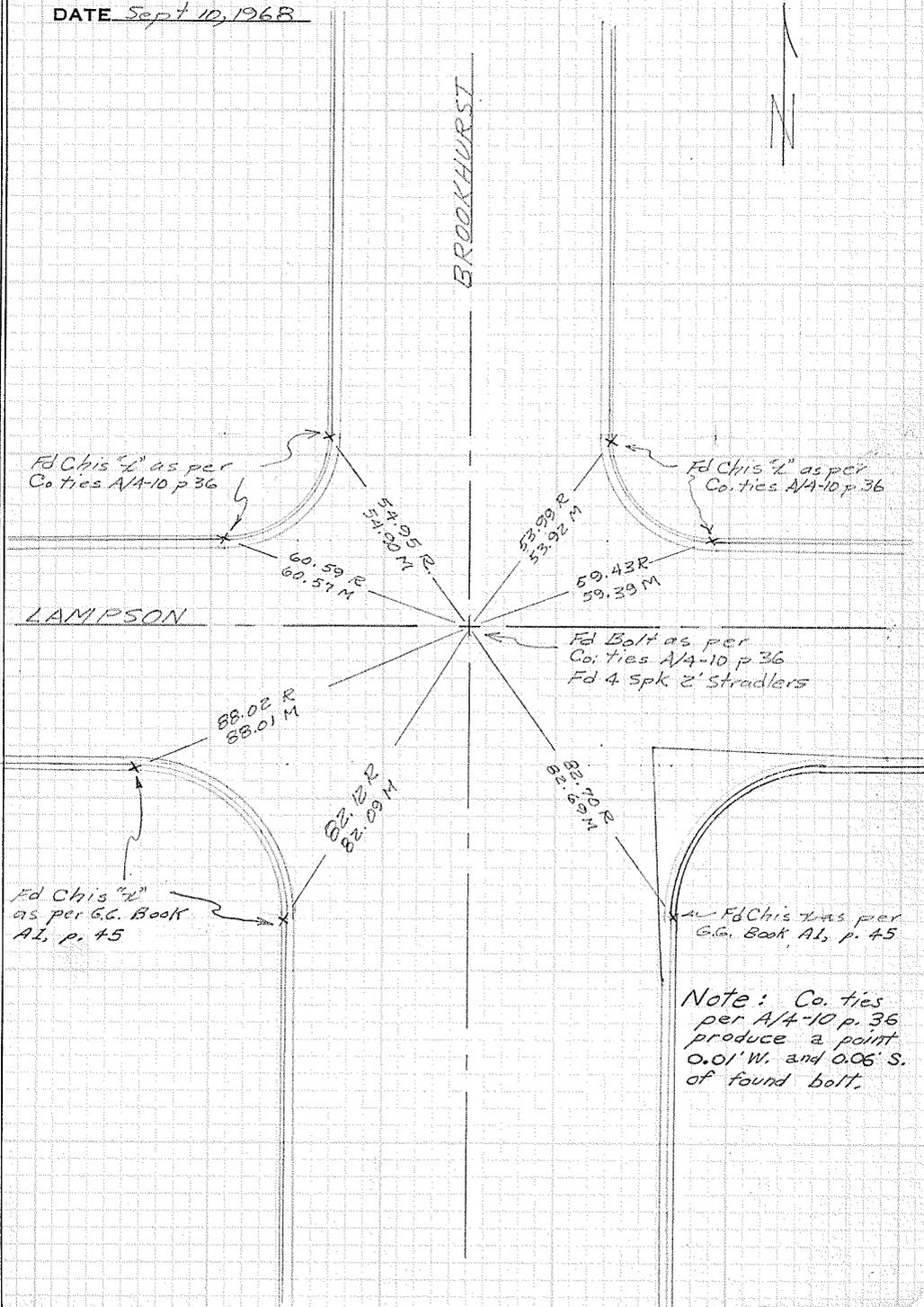
Note: Co. ties per A4-10 p. 36 produce a point 0.01' W. and 0.05' S. of found bolt.
